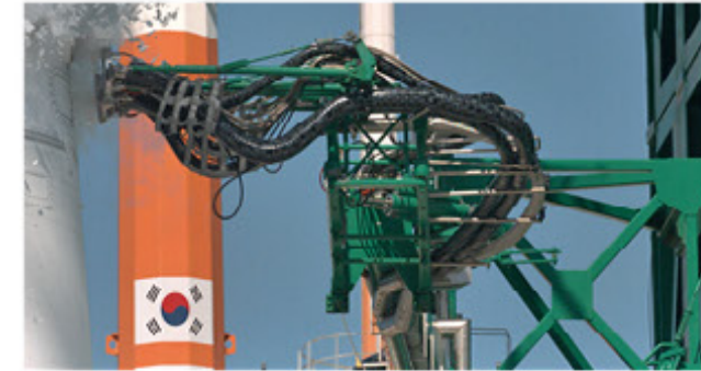
Scene of the Umbilical Device Separation During the Liftoff Moment of Nuri (KSLV-II)
